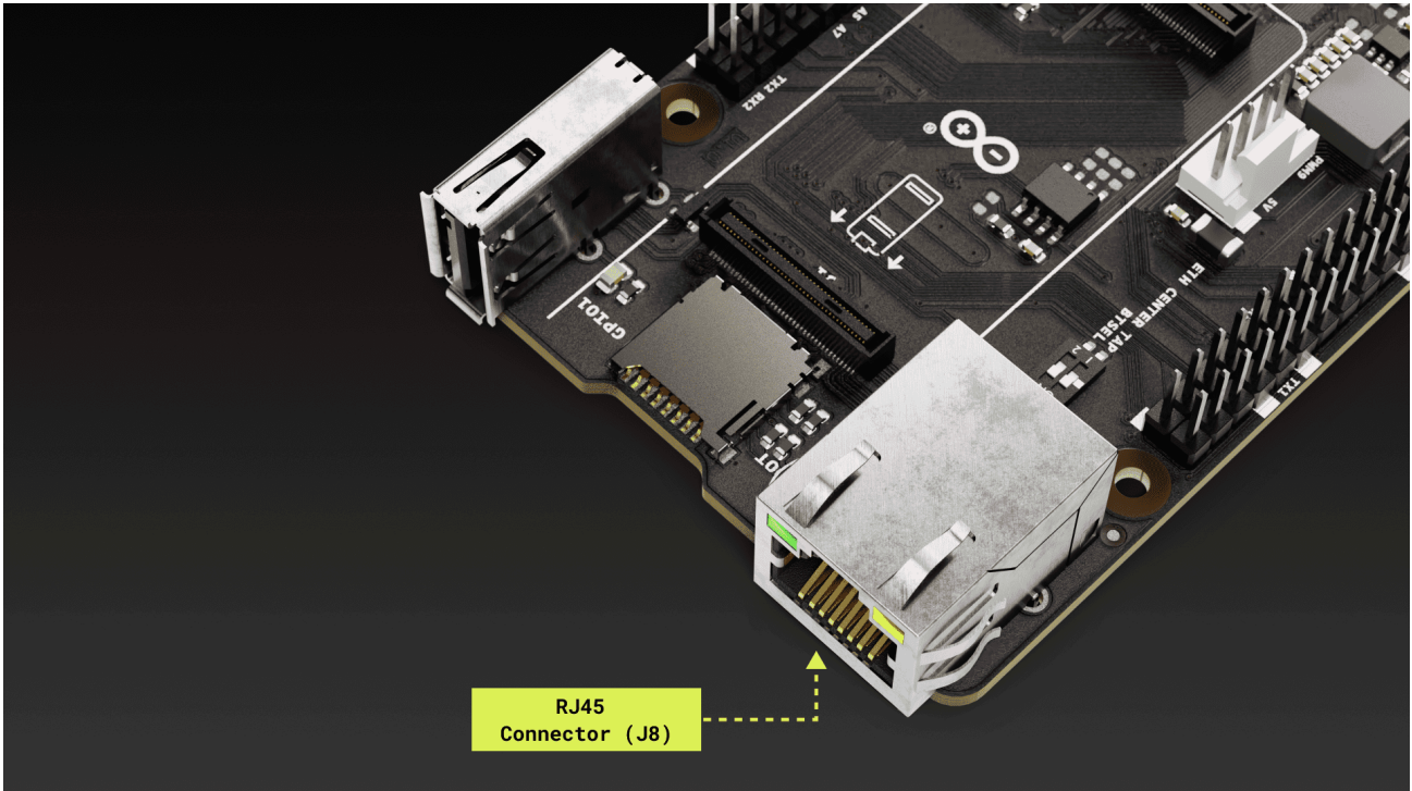
Figure 11. RJ45 connector of the Portenta Hat Carrier
